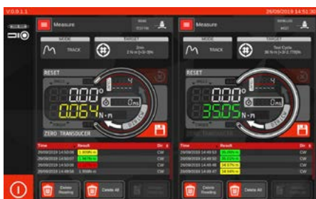
Displaying 2 transducer readings simultaneously
